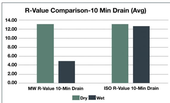
In the dry state, the measured average R-values were in line with published R-values for both the 2" ISO (R-13) and 3" Dual-Density Mineral Fiber (R-12.9). In the wet state, test averages again resulted in the polyiso product performing within percentage points of published R-values. In the same wet state, test averages resulted in the mineral fiber product R-values being diminished by 62% from published R-value.
