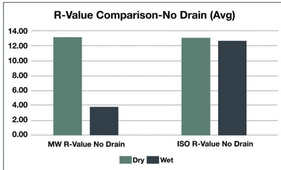
In the dry state, the measured average R-values were in line with published R-values for both the 2" ISO (R-13) and 3" Dual-Density Mineral Fiber (R-12.9). In the wet state, test averages resulted in the polyiso product performing within 3% of published R-values. In the same wet state, test averages resulted in the mineral fiber product R-values being diminished by 70% from published R-value.
