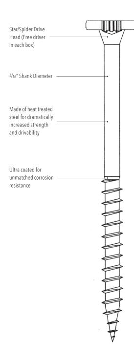
Hunter Xci SIP/WD Fastener is intended to mechanically attached Hunter Xci NB, Xci Ply and Xci Ply Class A to wood studs or wood framing. They can also be used for concrete and CMU applications with pre-drilling. Hunter Xci SIP/WD Fastener has the following features:
